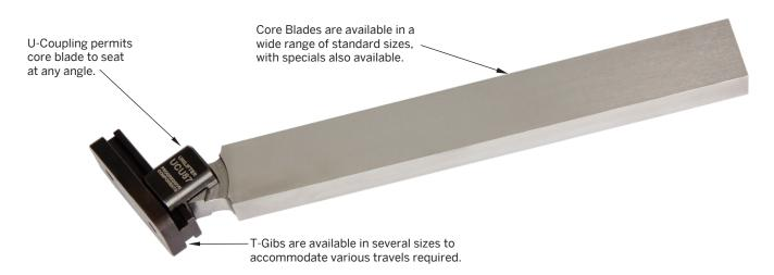
The UniLifter undercut release system incorporates a three piece set: Core Blade, U-Coupling, and T-Gib.
